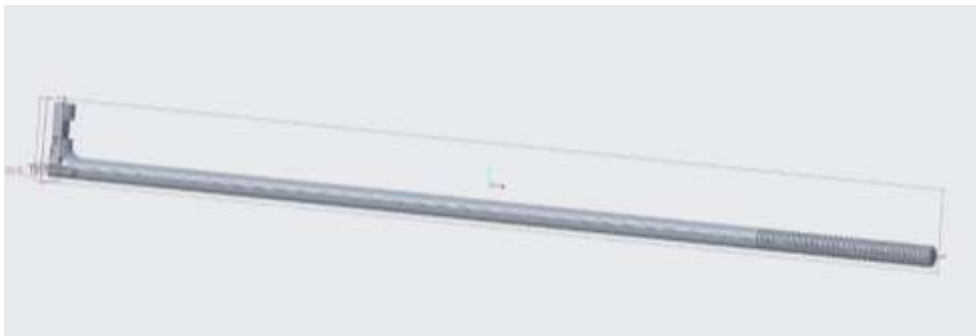
Fig. 2 :Battery clamp hold down rod designed in Creo.
