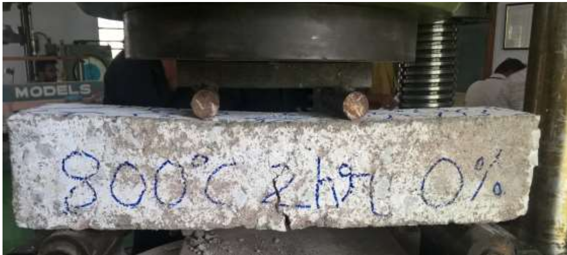
Figure 7: A view of beam specimen subjected to 800°C.
