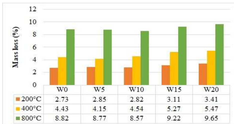
Figure 9: Variation of mass loss (%) of concrete with targeted temperatures
