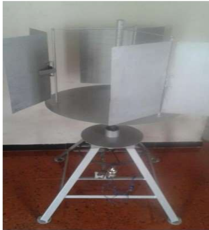
Fig 4. Fabricated butterfly bladed wind turbine
