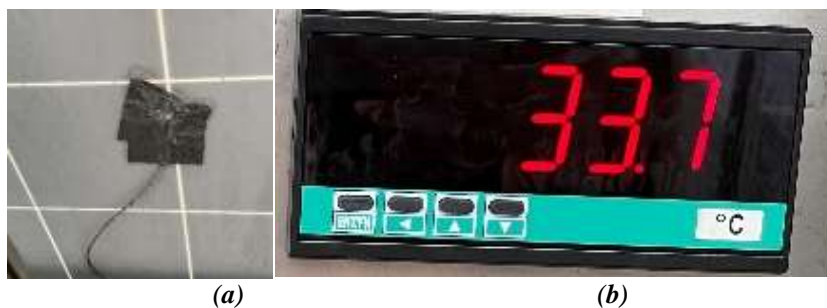
Fig. 3 Solar temperature monitoring device (a) Pt100 thermometer (b) digital electric meter
