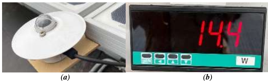
Fig. 2 Solar radiation monitoring equipment (a)pyrheliometer (b) digital electric meter
