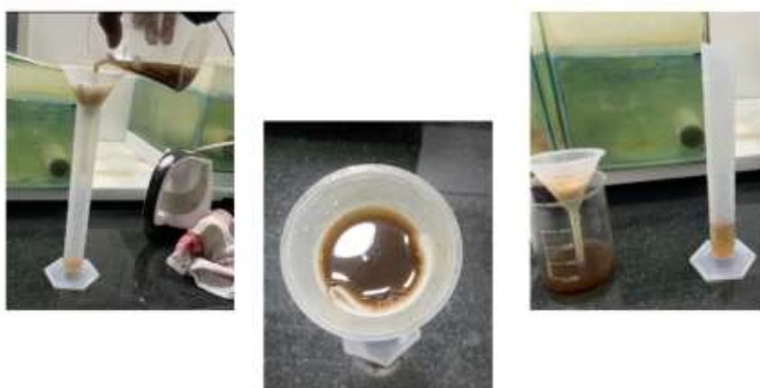
Fig 4: The extract was filtered using Whatman filter paper no.1 on a buchner funnel.
