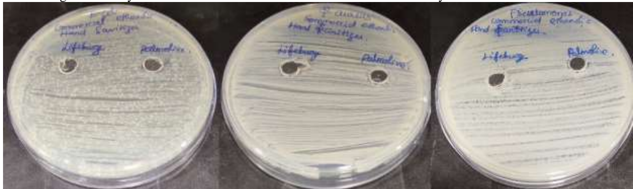
Figure 3: Analysis of zone of inhibition to evaluate antimicrobial efficacy of Alcohol hand sanitizers.
