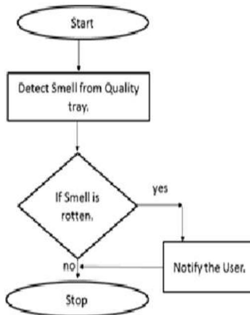
*Fig. 5 Quality Monitoring Flow using Smell Sensor*
