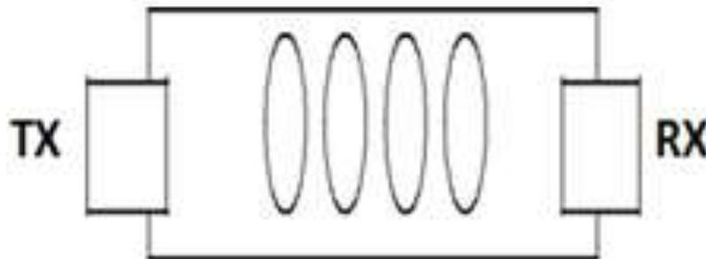
*Fig. 2 IR Sensor configuration when item are present*
