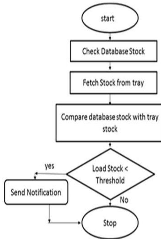
*Fig. 4 Quantity Monitoring Flow using Load Cell*
