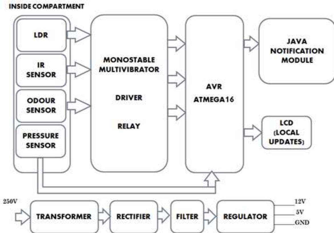
*Fig. 1 Block diagram of the Smart Refrigerator*
