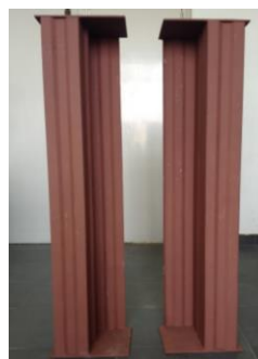
Fig. 5. Typical Z-section column with and without lip (1200mm)
