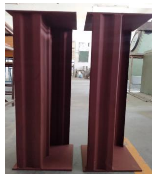
Fig. 4. Typical Z-section column with and without lip (600mm)
