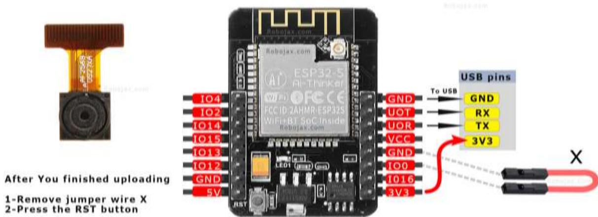
Figure 2 ESP32S Camera module
