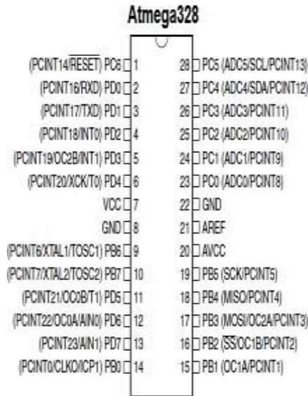
Figure 4 Pinout ATmega48PA/88PA/168PA/328P
