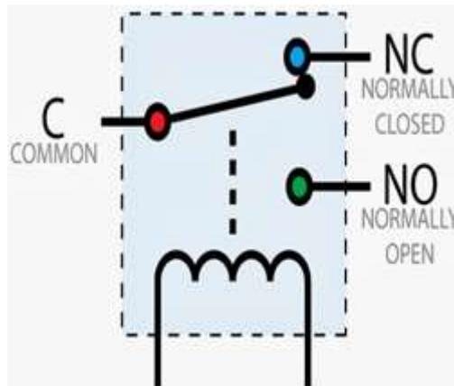
Figure 10 Relay circuit
