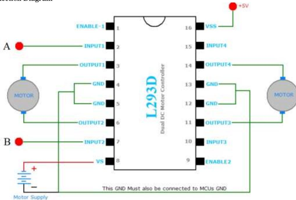
Figure 8 Connection diagram
