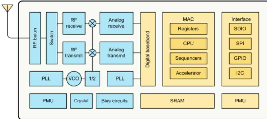
Figure 6 ESP8266EX block diagram
