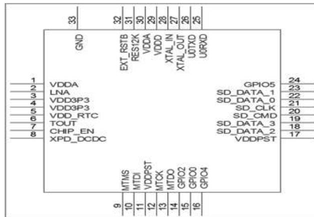
Figure 7 ESP8266EX pin assignments
