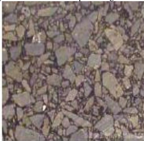
**Figure:1.1.Dense graded HMA**
