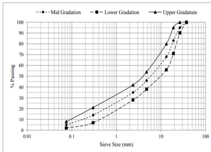
**Graph:3.2. Aggregate Gradation of Dense Bituminous Macadam (DBM) Mix**
