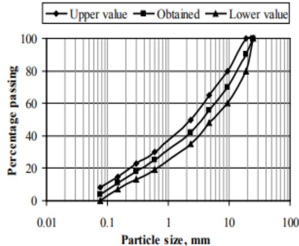
**Figure:** 3.5..Grain size distribution of aggregate gradation
