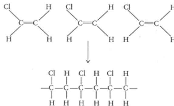
PVC consists of polar molecules which are attracted to each other by dipole-dipole interactions due to electrostatic attractions of a chlorine atom in one molecule to a hydrogen atom in another atom:
