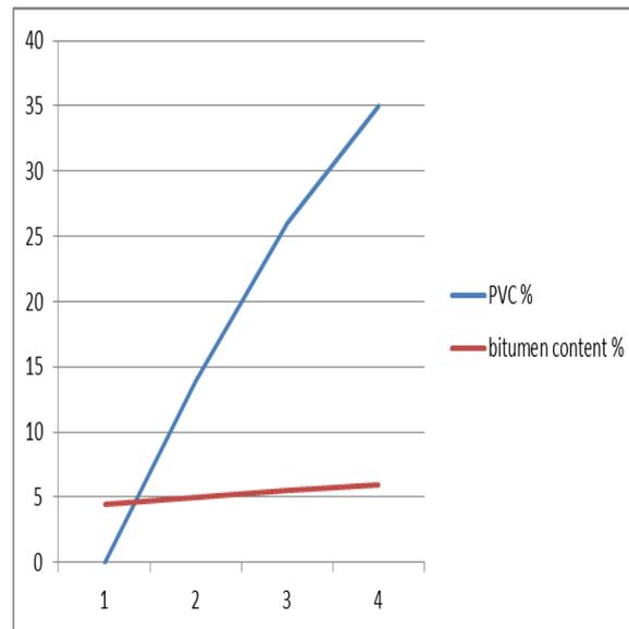
**Graph:4.4.Variation of PVC value with bitumen content at different coal ash content PVC with Bitumen:**
