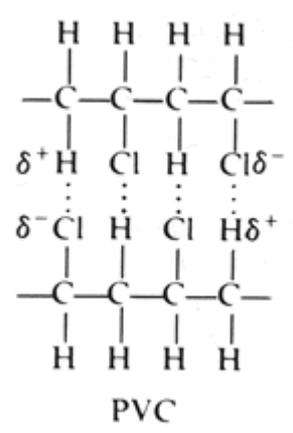
Polyvinyl chloride (PVC) is a popular thermoplastic that contains high levels of chlorine which can reach up to 57%. Carbon, which is derived from oil or gas is also used in its fabrication. It is an odorless and solid plastic that is white, brittle and can also be found on the market in the form of pellets or white powder. PVC resin is often supplied in the powder forms and its high resistance to oxidation and degradation make it possible to store the material for long periods. Some
