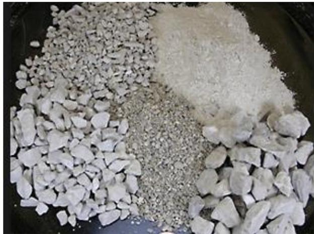
**Figure:3.4. Gradation of Aggregates**
