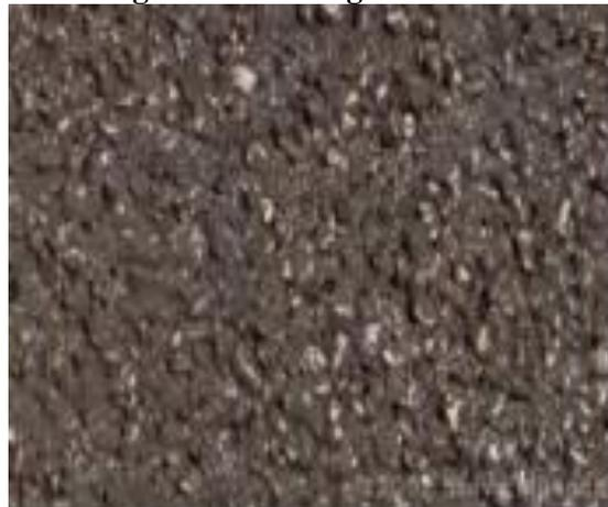
**Figure:1.2.Open graded HMA**
