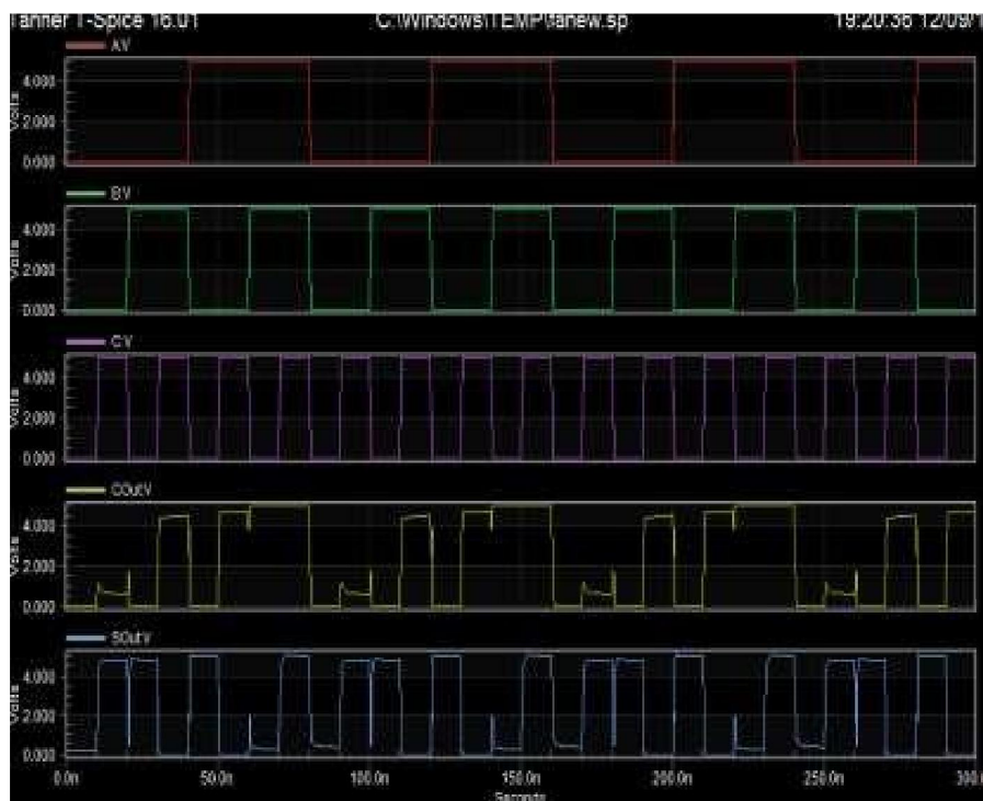
Fig.11. Proposed Full Adder Output
