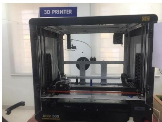
Fig 8. Fused Deposition Modelling
