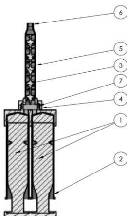
Fig 1. Design of Static Mixer
