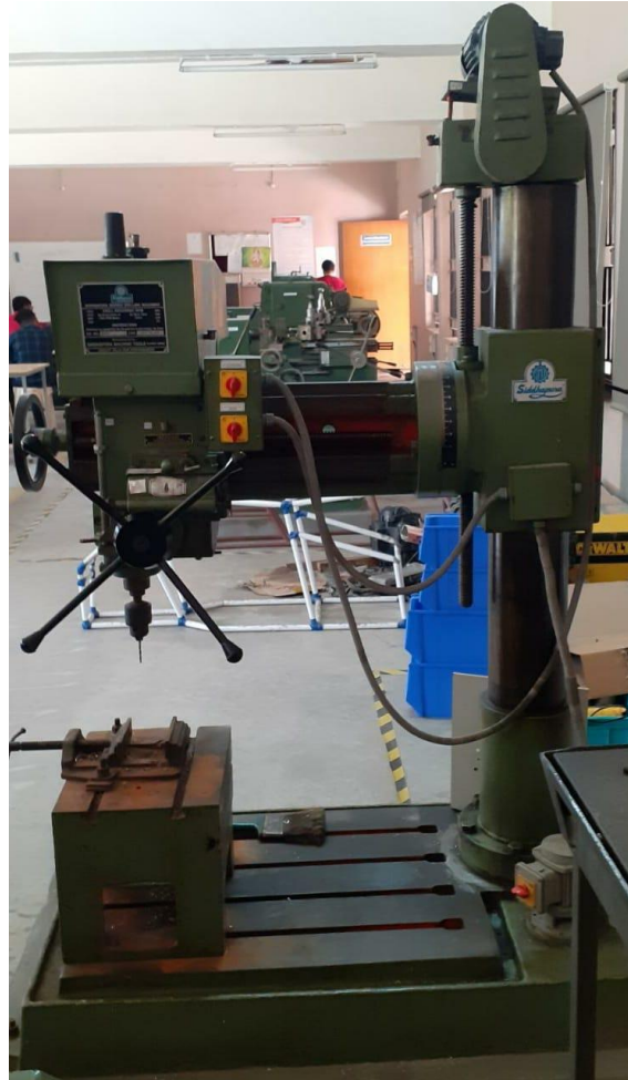
Fig. 3. Radial-drilling machine: Drilling capacity - \varnothing 25 mm. Table size - 400 mm, Range of the speed 2000-rpm, Feed Rate-0.5 -1.5 mm/min, Depth of cut - 0.3 to 0.7 mm, Tool diameter- 10 mm
