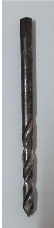
Fig. 2. The high-Speed Steel drill bit of \Phi 8\text{mm}
