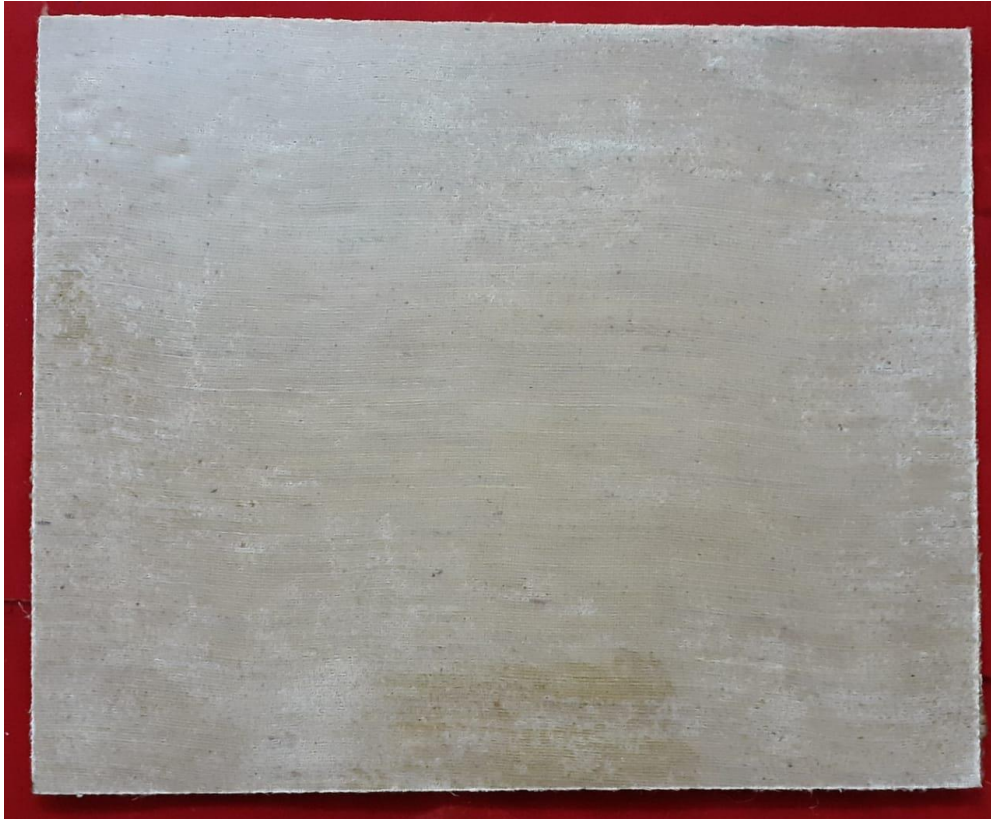
Fig. 1. Kenaf fiber Aluminium reinforced laminate of (300 X 300 X 5 mm) fabricated by hand layup technique
