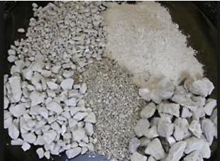
Figure: 3.4. Gradation of Aggregates
