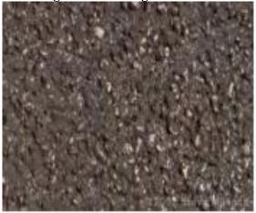
Figure:1.2.Open graded HMA
