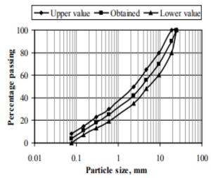
**Figure:** 3.5..Grain size distribution of aggregate gradation
