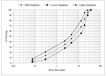
Graph:3.2.Aggregate Gradation of Dense Bituminous Macadam (DBM) Mix Preparation of Marshall Specimen:
