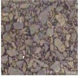
Figure:1.1.Dense graded HMA
