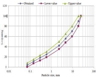
**Graph:3.3.** Grain size distribution of aggregate gradation
