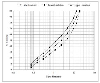
Graph: 3.1. Aggregate Gradation of Bituminous Concrete (BC) mix
