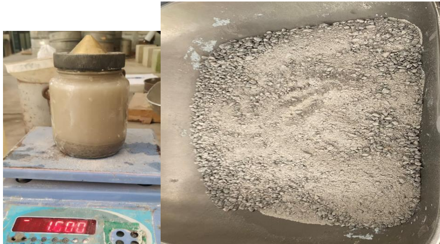
Fig. 2.3.4 Pycnometer with wet Stone Dust and Stone Dust in a try
