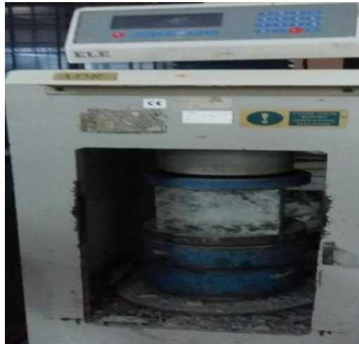
Fig. 2.9. Compressive Strength Test
